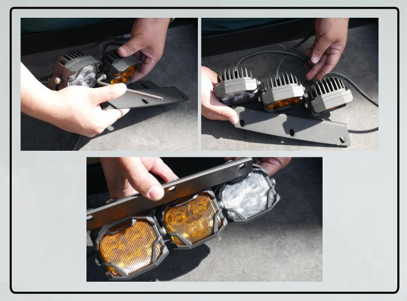
11. Using a Tp40 (Torx Plus) socket or L-Key, remove the 3 bolts on the bumper and reinstall through assembled 4Banger bracket.
