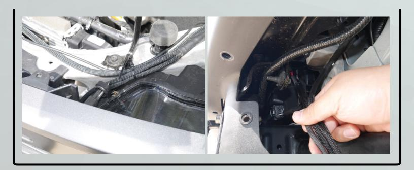
8. Optional: Bumper end cap can be removed for additional space during installation. To remove, pull push pins out of the plastic cover surrounding the tow hook.
