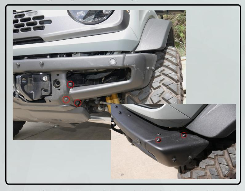
10. Begin assembling the pods and brackets. Fit the square shoulder carriage bolts as shown. Fit the Torx T30 screws but do not fully tighten yet.
