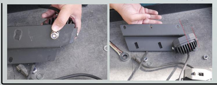
Pods should be mounted from outside-in, tightening the pod adjustment screws after installed (access becomes tight when all pods are mounted)
