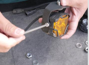
NOTE: Pod should be mounted in the same direction as the slots (bracket should be close to parallel)
