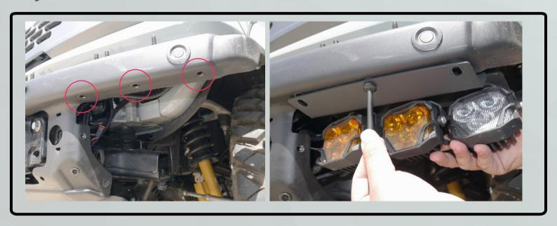
12. If the bumper caps were removed, they can be reinstalled in the reverse process of removal.
