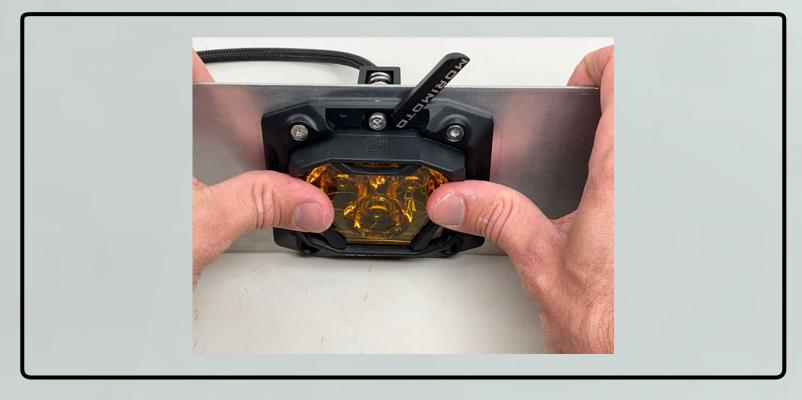
12. Finally, insert the bottom two front bezel to mounting bracket screws and tighten all four screws. Use the adjuster screw to aim the pod to your desired vertical angle. Tightening this screw will adjust the pod to aim higher, loosening will aim down.
