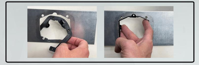
6. Align the front bezel to the same mounting holes and, using a Torx T20 bit, loosely install the top two M4 x 22mm flat head screws (note that the bottom two screws will be installed later.) Leave these top two screws finger tight.
