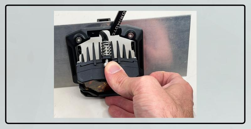
10. Open the adjuster door on the front bezel. Making sure that the spring does not fall off the back of the screw, insert the pod through the bezel and onto the mounting bracket. Get the adjuster screw started into the adjuster threading clip. Turn the adjuster screw 5-6 turns but do not tighten down.
