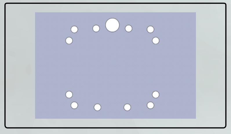
3. Using a Dremel or cutoff wheel, "connect the dots" of the inner 0.25" / 6mm holes. Be careful not to intersect the four outer mounting holes. Try to cut along the outside wall of these holes.
