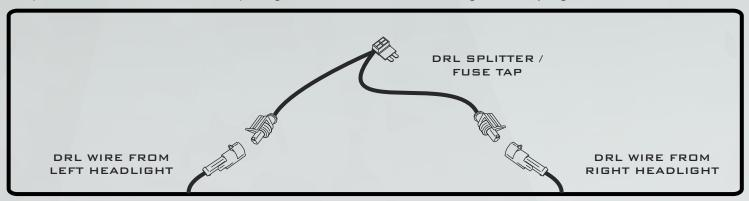
11. (OEM HALOGEN TRUCKS ONLY): Route the DRL "Y-Harness" across the top of the radiator support and the fuse tap to the fusebox. Insert the fuse tap into position #35 as indicated.
