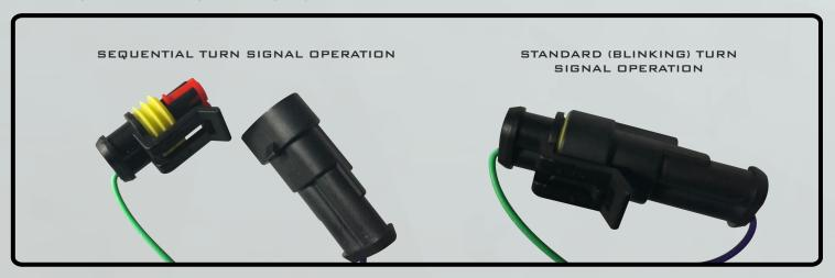
18. Test all functions of lights before bolting them on to the truck. We recommend leaving the lights on for five minutes with the truck's engine running. Certain functions require the capacitors to have a charge which naturally takes a short amount of time.
