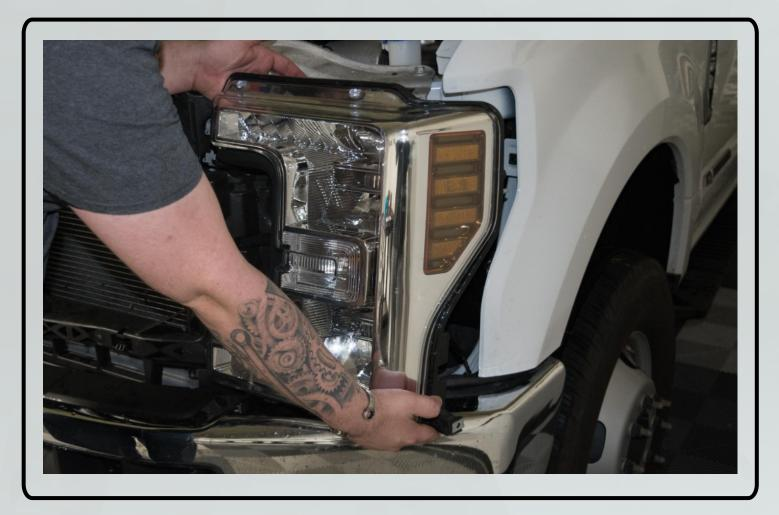
8. Unplug and remove each electrical connection from the back of the housings. For the halogen trucks, there are four electrical plugs to remove from the back of each housing.
