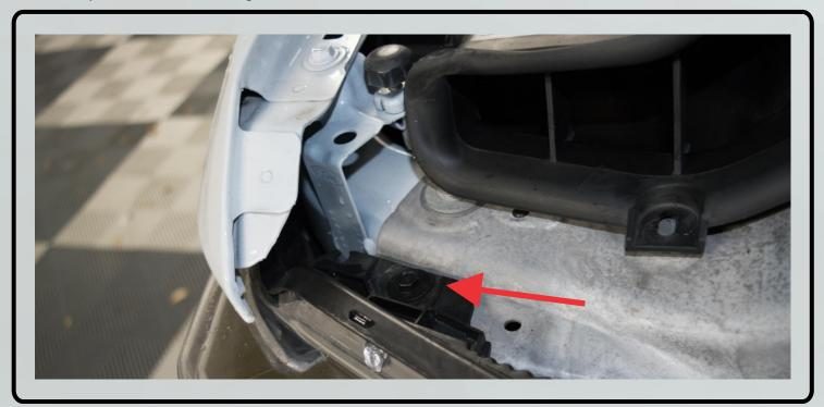
6B. The most difficult bolt to access is indicated. It is best removed with patience and a ratcheting 10mm closed-end wrench and is accessed via a very slim opening between the fender liner and bumper. There is one of these bolts per headlight (two total).
