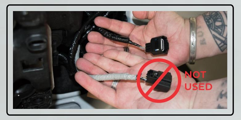
10. (OEM HALOGEN TRUCKS ONLY): Plug in DRL leads to each headlight's DRL plug
