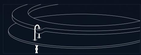
Place a bead of RetroRubber sealant in channel of headlight housing as shown. Fill the majority of the channel to ensure it sufficiently holds the front lens once re-installed.
