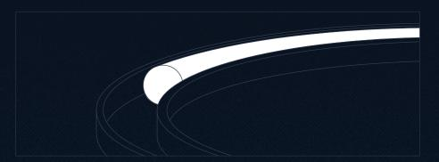
Use scissors to cut the RetroRubber once the entire circumference of the housing has been filled.
