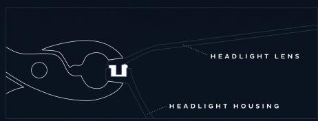
Allow thirty (30) minutes for headlight to sufficiently cool down prior to re-installation on car.
