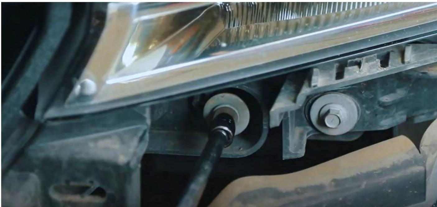
Detach the plastic clips that secure the light wiring.
