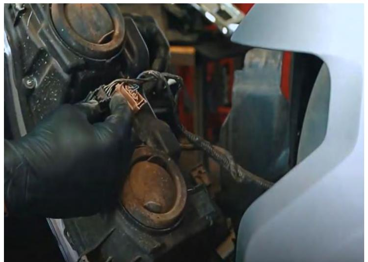
Disconnect the wiring connection from the back of the headlight housing and place it aside.
