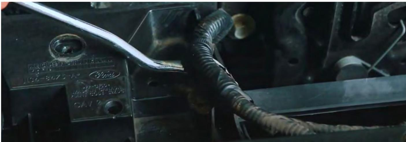
Disconnect the two connections for the active grille located at the top of the radiator area.
