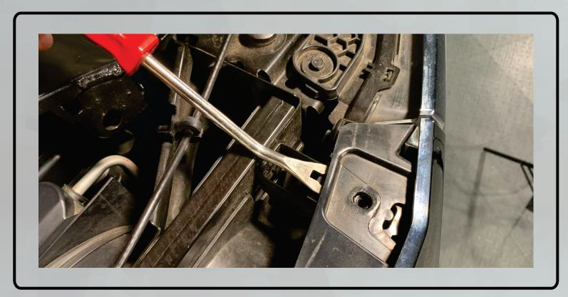
4. To remove the grille, firmly pull forward to release the push clips.
