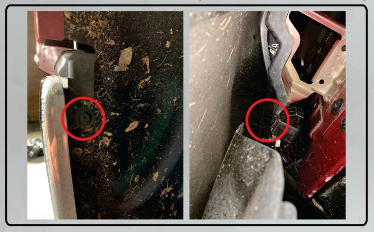
8. Back on top, use a trim tool or flathead screwdriver to pop the headlight bracket up and off of the slot in the fender retaining it.
