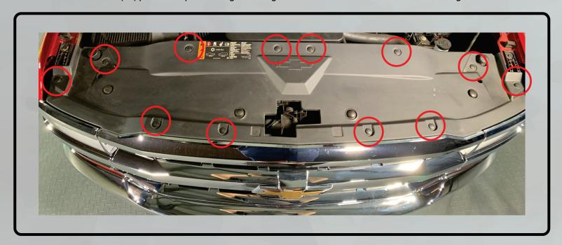
2. Remove the four (4) 10mm bolts holding the grille to the truck.
