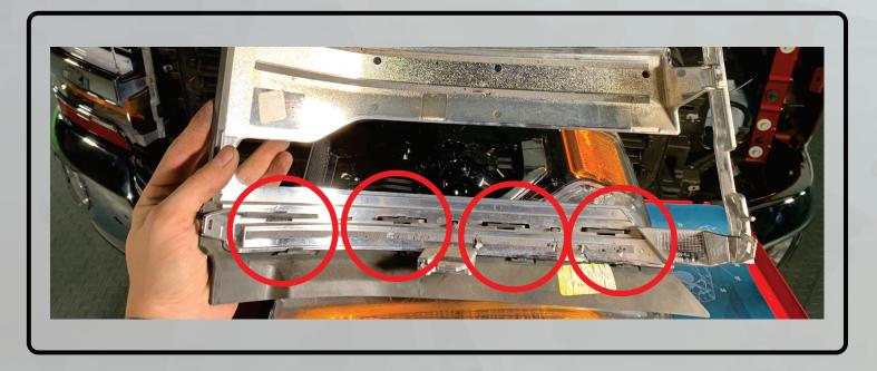
13. With the provided alcohol wipes, clean the indicated areas of the back of the trims and corresponding locations on the headlight assemblies.
