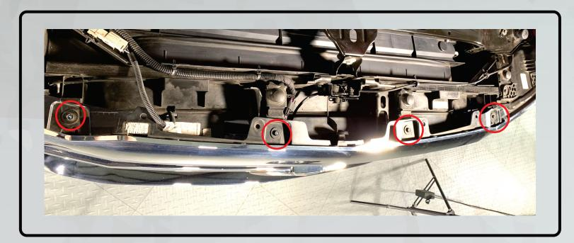
3. Using a trim tool or flathead screwdriver, pop the grille up and off of the tabs where the bolts were previously installed.
