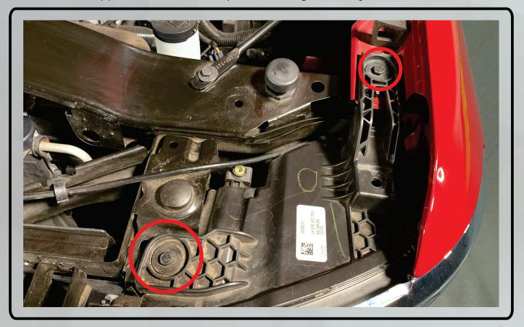
6. Remove the 10mm bolt from the bottom of the headlight behind where the stock grille was.
