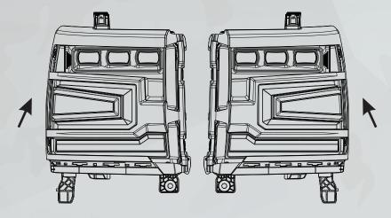
15. Click in the factory painted trims at the bottom of each headlight to attach.
