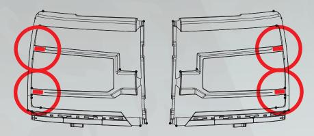
14. Adhere the double-sided foam adhesive pieces to the cleaned locations in step #13. Fit the trims to the front of the headlight and press gently to attach.
