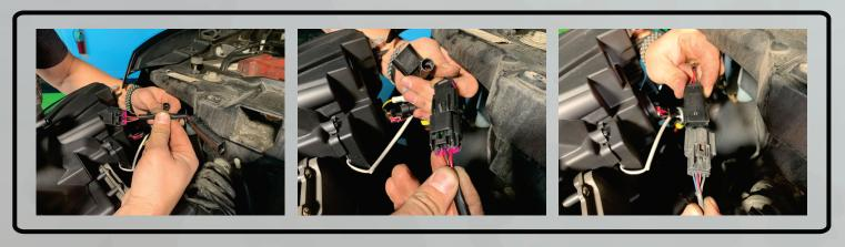
8. Connect the turn signal connector to the factory turn signal plug.
