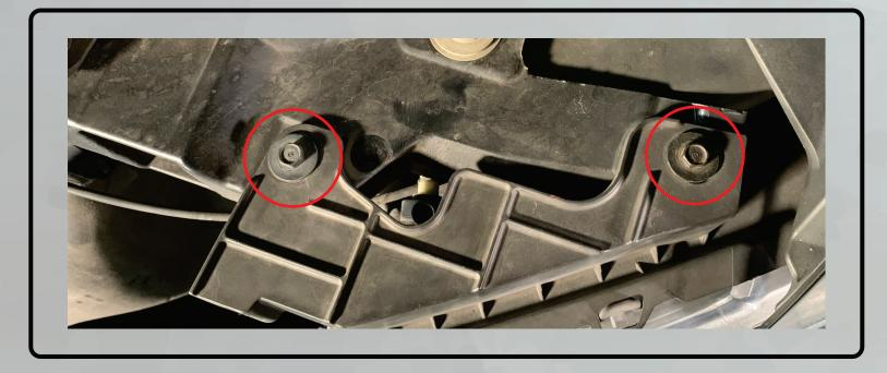
4. Using a trim tool, pop the headlight's ball joint out of the fender clip near the side reflector.
