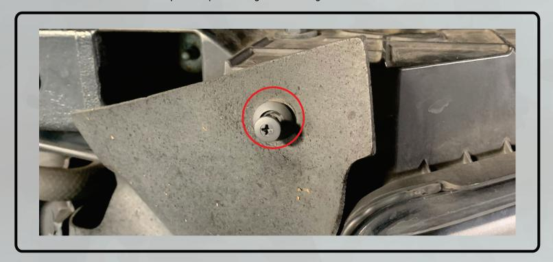
2. Remove the 10mm bolt retaining each headlight behind the grille surround.
