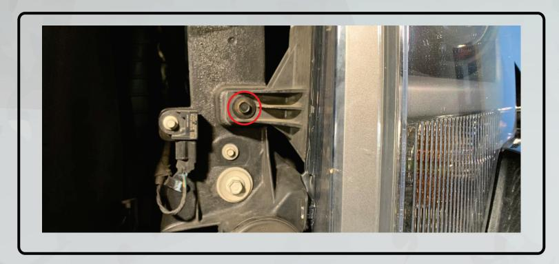
3. Unscrew and remove the two 10mm bolts retaining the top of each headlight.
