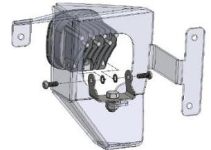
6. Place the new fog pocket assembly over the three circled mounting holes below and thread in the OEM screws. Tighten the fasteners. Plug the harness adapter into the OEM harness and into the Squadron power cord. Lock the OEM connector. Repeat for the opposite side.
