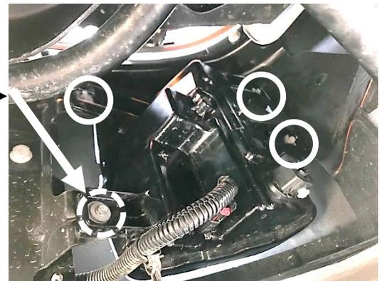
5. Locate the hardware bag. Use the 9/16" hex head hardware to attach the Squadron bracket to the fog pocket mount (see passenger side exploded view below on the left for reference). Now, using the 4mm Allen head hardware, place the light onto the Squadron bracket through the front opening of the fog pocket mount (See exploded view on right below). Repeat for the opposite side.
