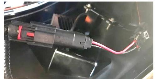
7. Tie all wires away from any hot or rotating components. Reattach battery.
