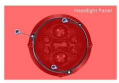
**Figure 5:** Secure the light to the mounting ring using the supplied trim ring and three 8x32 x ¼" phillips screws.
