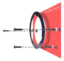
**Figure 2:** Insert a ¼ x 1.5 in. screw through the mounting ring hole, then through one of the supplied springs and then into the headlight panel hole.
