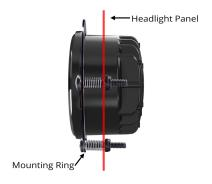
**Figure 7:** Tighten the three Torx screws until the springs are compressed approximately halfway. If there is an obstruction, back out all three screws about ¼ inch.
