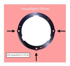
**Figure 1:** Using the mounting ring as a template, use a 6mm or ¼ in. bit to drill three holes in the vehicle's headlight panel.
