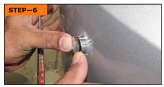
Insert the parking sensors into the bumper, ensure the ridge is at the top
