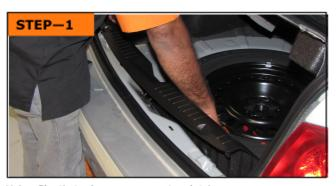
Using Plastic tool, remove rear trunk trim.
