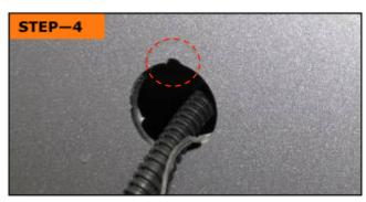
File a small gap at the top of the hole, so that the ridge of the parking sensor fits well and will not move.
