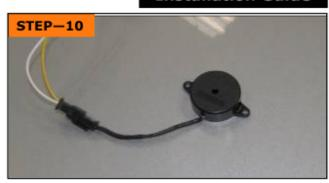
Connect the buzzer. Using the double sided tape, place buzzer in the trunk, in a hidden position. Position the buzzer so it can be heard well from the driver seat.
