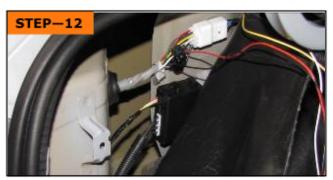
Use double sided tape provided to secure the module, and secure all wires with cable ties..
