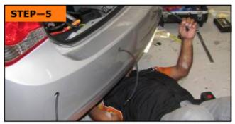
Pull SP4 loom through the holes in the bumper, as shown. Connect to the sensor heads. Secure SP4 loom with cable ties
