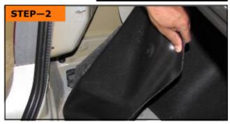
Using plastic tool, remove left side interior panel to reveal reverse light connection.
