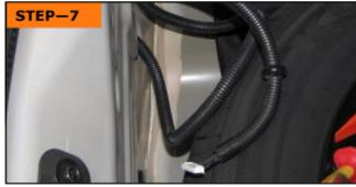
Pull SP4 loom (module connector) through grommet underneath the trunk floor and into trunk cavity.
