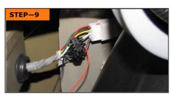
Use the quick connector to connect to reverse light power and ground.
