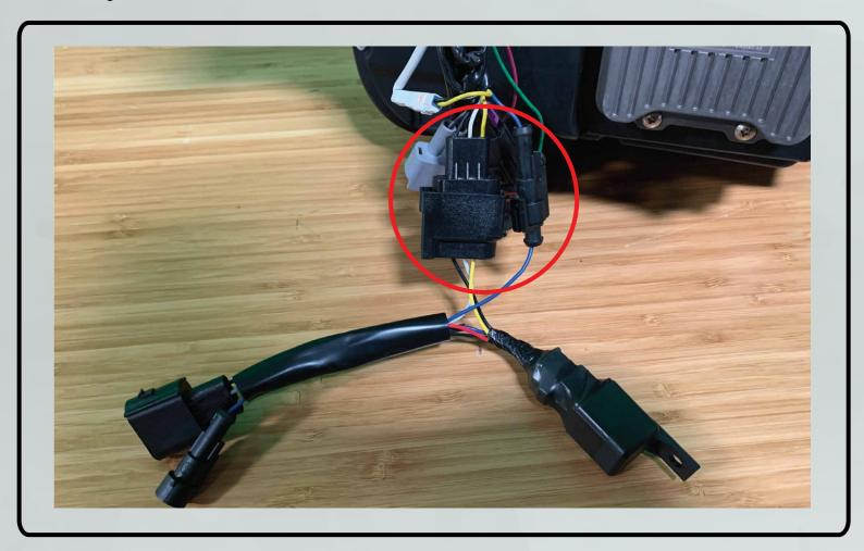
3. Plug these connectors (#1) into the truck harness and mount the relay (#2) to secure it.
