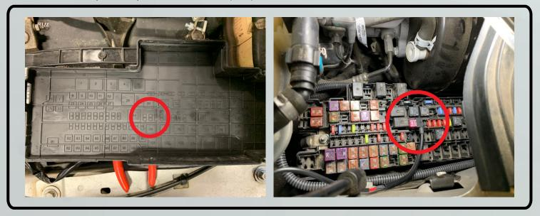
7. Connect XB LED headlight to factory headlight connectors.
