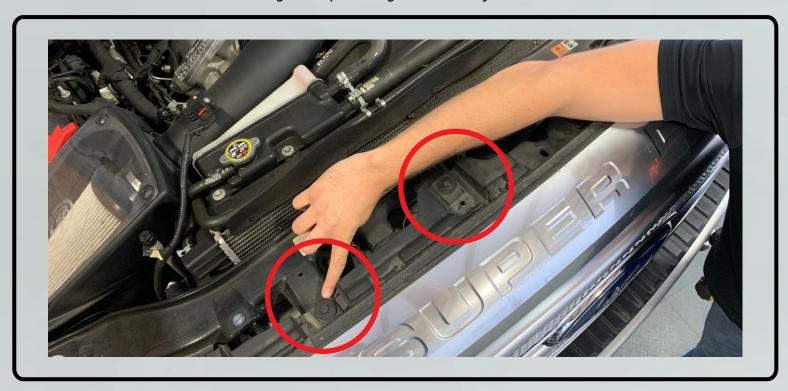
2. Use a long flat-head screwdriver to depress the five clips at the bottom of the grille shell to release it.
