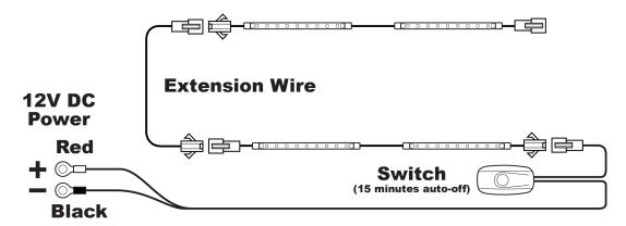
2. **Mount the lights:** Place one LED string on the left side of the pickup truck bed and the other LED string on the right, and connect them with the extension wire. Clean the mounting surface. Use the
